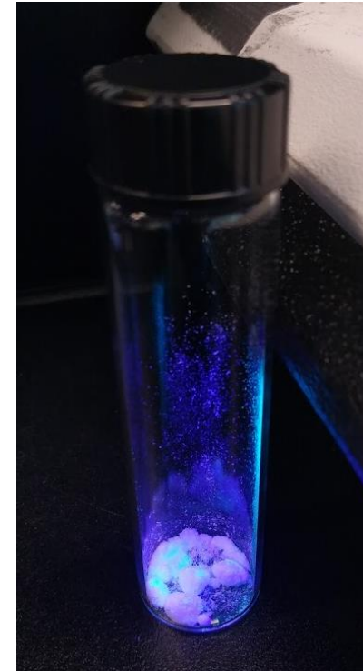
SFS is fluorescing in solid state, PPO is not
