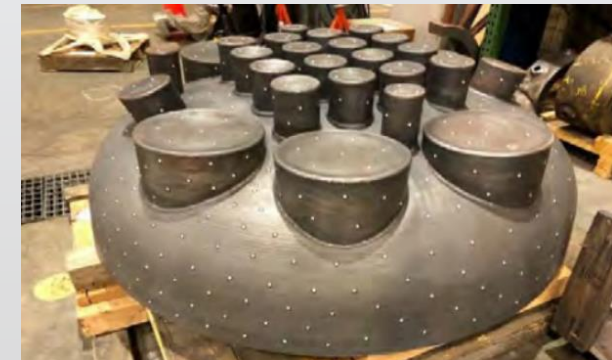
Powder Metallurgy - HIP Hot Isostatic Pressing 100 to 10,000 lbs
