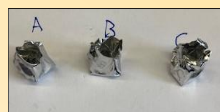
Figure 2: PuO 2 powder wrapped in Al foil (left) and neutron flux monitors mounted onto quartz tubing (right).
